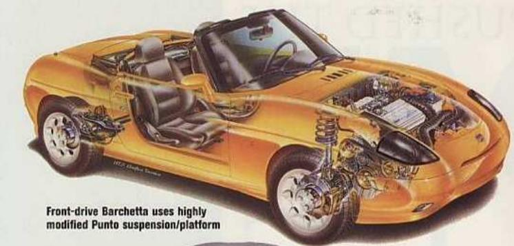
Front-drive Barchetta uses highly modified Punto suspension/platform
