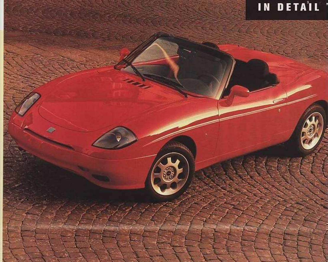
Small bonnet and boot on voluptuous Barchetta a contrast to Fiat Coupe's, though its separate square rear lights make link with Coupe's circular items. Wheels are a '90s interpretation of a '60s theme and unusual door handle based on '50s cars like 8V. Mirror and internal door treatment decidedly '90s
